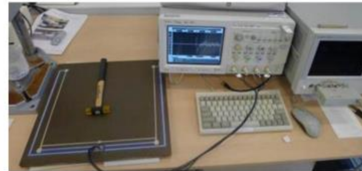
PiezoPaint™ based distributed network of sensors printed onto CFRP plate
