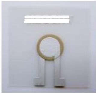
PiezoPaint™ based test sample printed on Polyester substrate
