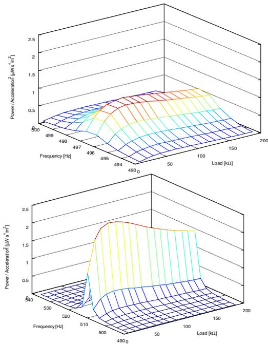
Fig. 3. Normalised power output (RMS) as a function of the excitation frequency and resistive load, for 12.5x2 mm<sup>2</sup> structures based on standard PZT (top) thick film and high-performance thick film (bottom).
