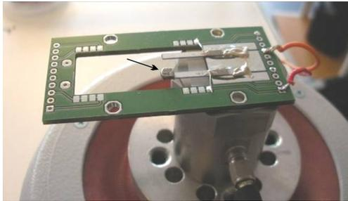
Fig. 2. Measurement setup, showing the test fixture with two cantilevers mounted on the shaker system, one of them with visible clamp-on seismic mass.
