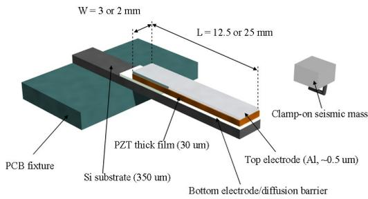
Fig. 1. General structure of the cantilever-shaped energy harvesting generators.
