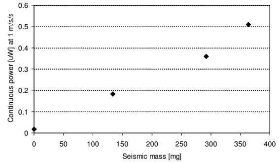
Fig. 4. Output power vs. seismic mass at 1 m/s<sup>2</sup> of bending element based on PZT standard thick film.
