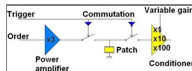
Fig. 11. Structure of a channel of the LWDS45-2.
