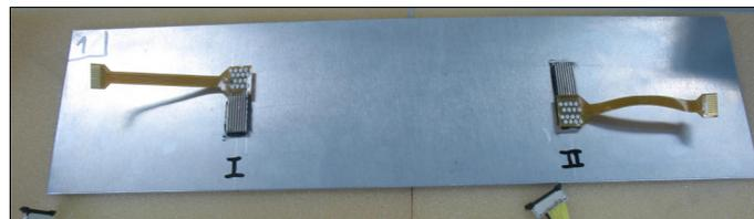
Fig. 8. Picture of an aluminum test plate with integrated piezo-composite patches.
