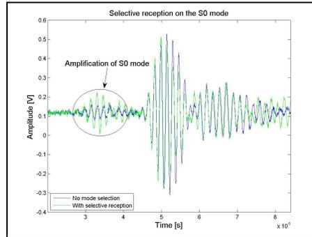
Fig. 14. Performance of the selective reception technique with the  $S_0$  mode.
