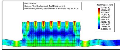
Fig. 3. FEM model of the piezo-composite patch.
