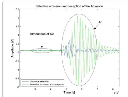
Fig. 18. Performance of the mode and direction selection techniques with  $A_0$  mode.
