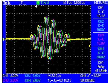
Fig. 16. Four excitation signals to obtain selective emission.
