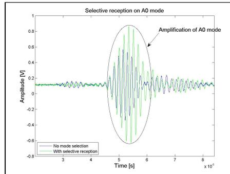
Fig. 15. Performance of the selective reception technique with the  $A_0$  mode.
