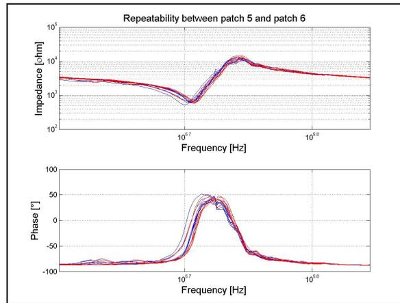
Fig. 6. Frequency response of the eight elements for the piezo-composite samples n°5 (blue curves) and n°6 (red curves).
