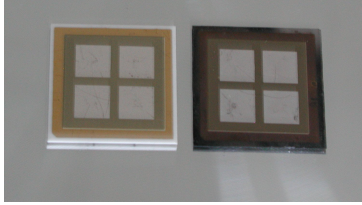
Fig. 2. A picture of the actual structure taken with a digital camera. Alumina substrate on the left and silicon substrate on the right. Each sample is 30x30 mm 2 .
