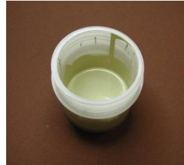
PZT powder is suspended in an organic vehicle
