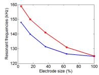
Fig 3. Evolution of the main resonant frequency versus the fractional electrode area.
