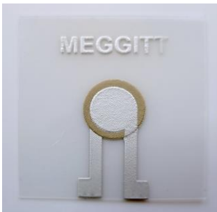
PiezoPaint™ based test sample printed on Polyester substrate
