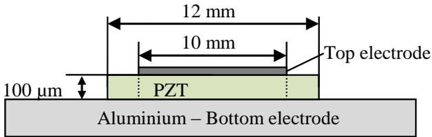
Figure 4. Cross section view of the PiezoPaint™ sensor.
