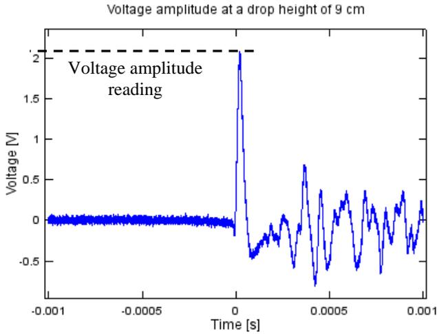
Figure 10. The measured voltage signal (9 cm drop).
