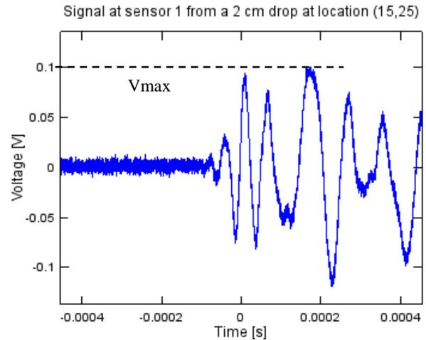
Figure 9. The voltage output at sensor one for a 2 cm drop. The maximum amplitude is 100 mV.
