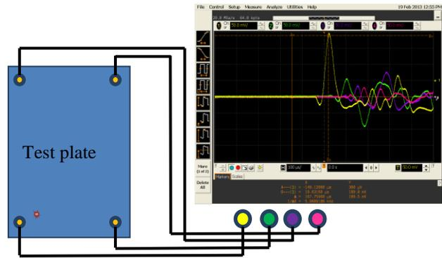
Figure 6. Measurement setup for impact detection experiments.
